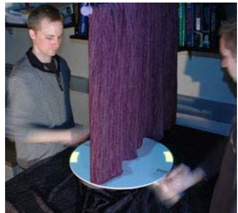
Author Kyle Reed demonstrates his apparatus for investigating haptic communication when two people try to complete a simple physical task together.
